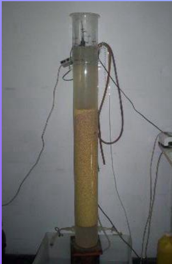
Reactor "air lift"
